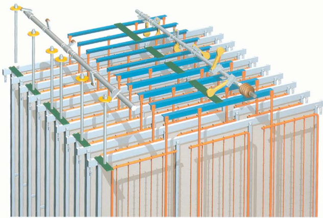
Electric corona discharge system (gas purification zone)
