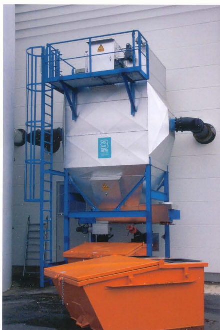
BETH small electrostatic precipitator Biomass incineration system, 9,600 m 3 /h < 50 mg /NNm 3 dry at 220° Celsius
